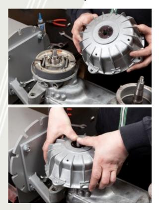
Step 5: When the settings are done, the hub can be fully fitted. Make sure you are using the wavy washer under The domed nut and also apply some Loctite to the allen screw holding the lock washer.
